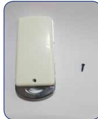
**EN** Use a screwdriver with a 1.2 mm tip to unscrew the back screw
