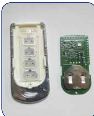
**EN** With the help of a coin, release the cover.
